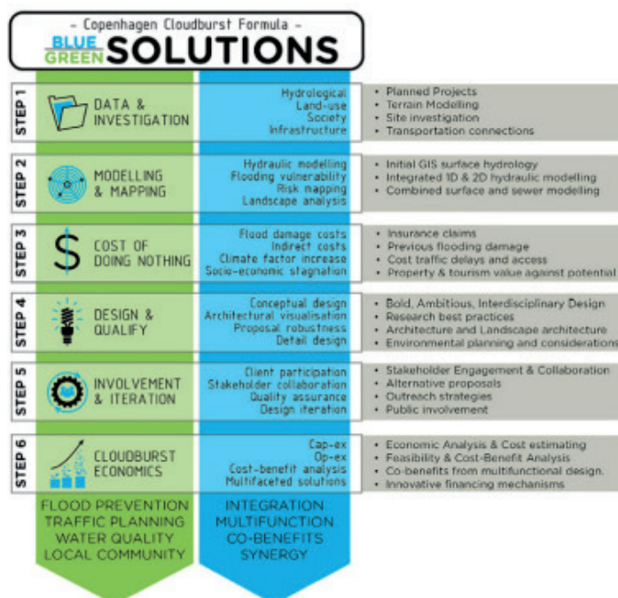
Figure 5.12. 6 step procedure for the integration of the Blue-Green Approach in Copenhagen Cloudburst Formula ( https://oppla.eu/casestudy/18017 )
