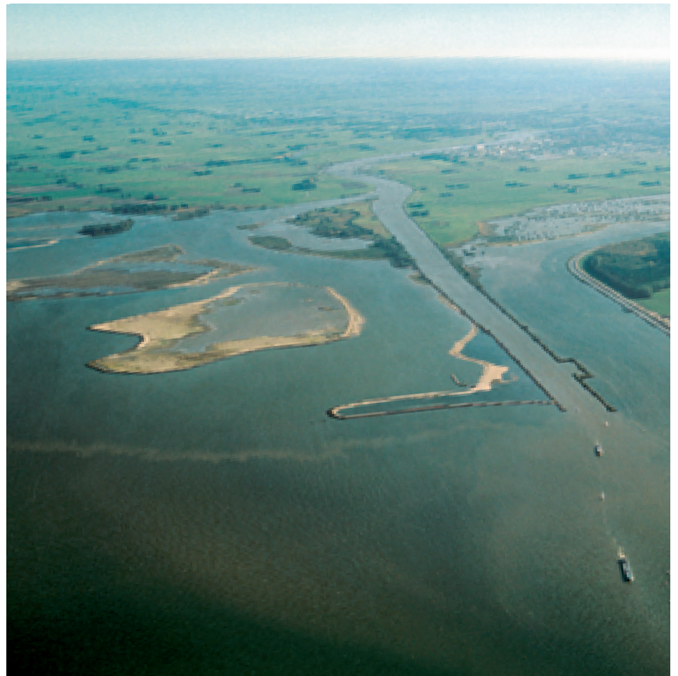
Figure 7. Also created from clean fill is an 800 ha nature reserve at the mouth of the IJssel (IJsselmonding).
