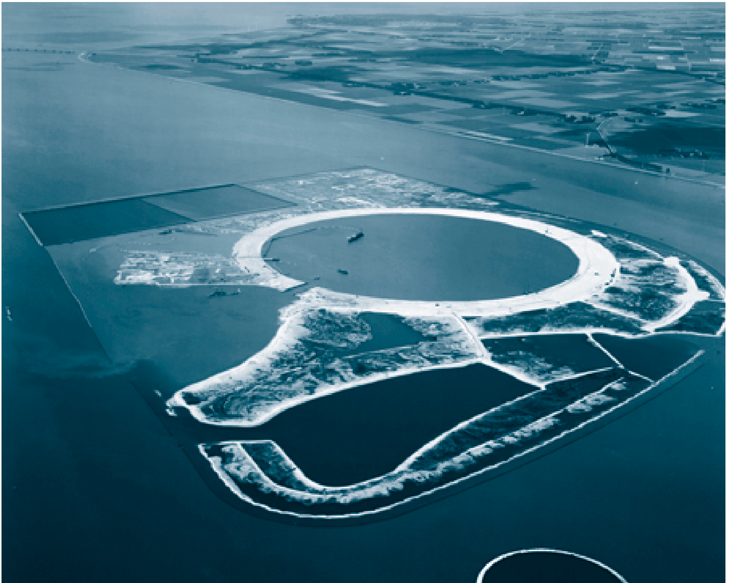
Figure 5. Where does the Water Framework Directive apply? In the northern Netherlands, a branch of the Rhine, the River IJssel, carried contaminated silt into Lake Ketelmeer where it settled into the bed. In an action to clean-up the waterway, the IJssel-oog (eye) repository was constructed for safe storage of contaminated dredged materials.
