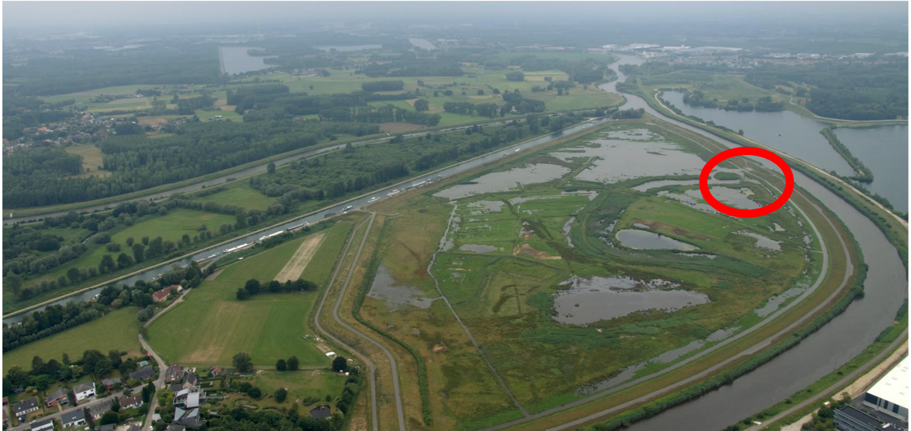
Innovative approach Controlled flood areas with reduced tides – Zennegat (Mechelen)
