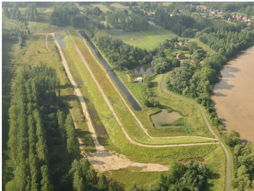
200.000 m 3 sediments used for a 2 km long floodbank
