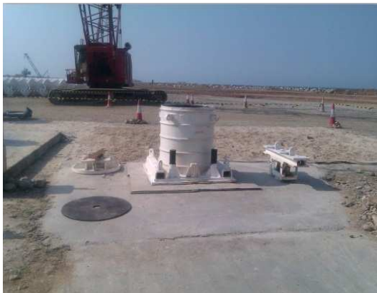
Calibration chamber equipment and sand spread out for drying
