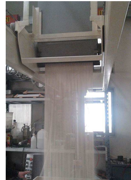
Pluvial deposition in air
